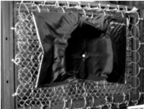
Schuss-Simulation – Aramitgewebe Impact simulation – aramid fabric
